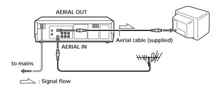
Disconnect the aerial cable from your TV and connect it to AERIAL IN on the rear panel of the unit.
